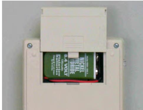
To gain access to the battery, the battery compartment cover must be removed as shown above.
