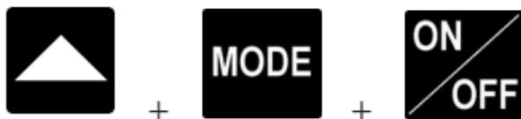
Turn the Microscanner Pro OFF, then hold the ▲ and MODE keys down while pressing the ON key to display your hardware and software versions.
