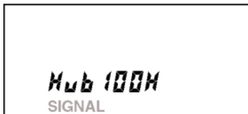
The word SIGNAL blinks once every two seconds below the word Hub. Go to the wiring closet to view a light that blinks once every two seconds at the port to which the cable is connected.
