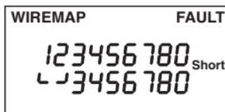
When the wiring fault includes shorted or swapped non-pair pins (that is, non-pair pins 1-3), the wiremap will display dashes for those numerical wire indicators.
