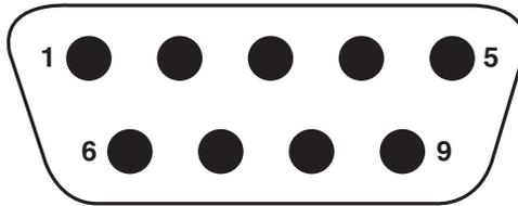
**Fig. B-1. Printer Connector.**
