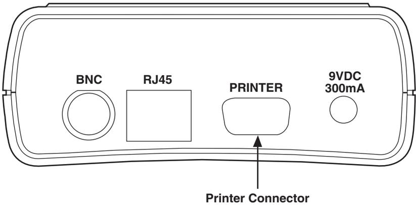
**Fig. 6-1. Printer Connector on the Scanner.**
