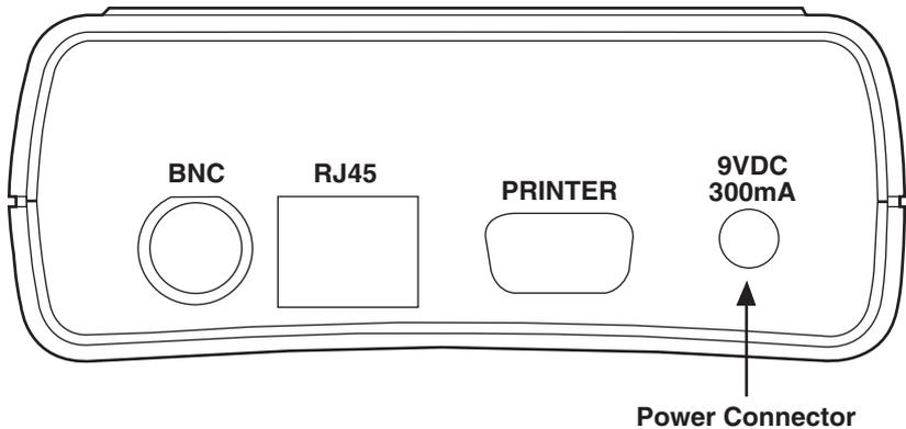
**Fig. 3-1. Power Connector on the Scanner.**
