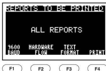
The serial-data format is fixed at 8-bit, no parity, 1 stop bit (8N1).
