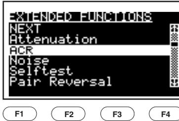
3. Press ENTER. The test begins scanning immediately. (Press the arrow keys to select another cable test standard.)
