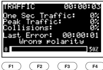
Figure 11-2. Traffic Test Results Screen (No Link Pulse).
