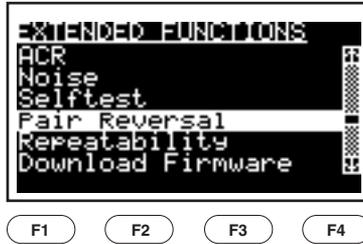
4. Press ENTER. Press ESC to abort the test. (Press the arrow keys to select another cable test standard.)
