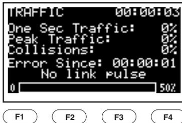
Figure 11-3. Traffic Test Results Screen (Jabber Detected).
