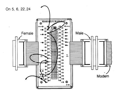
Figure 3. Modem Loopback Test
