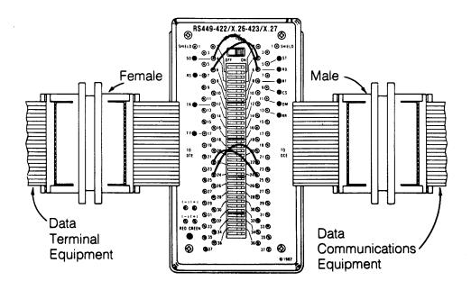
Figure 4. Null Modem Cable Interface
