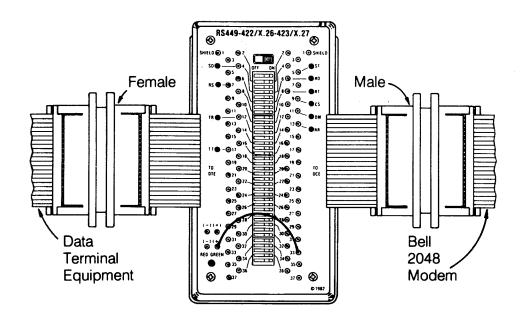
Figure 2. Checking EIA Signals
