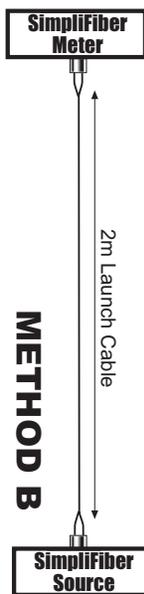
4. Power on the SimpliFiber Meter. The unit will auto-sense the appropriate wavelength.
