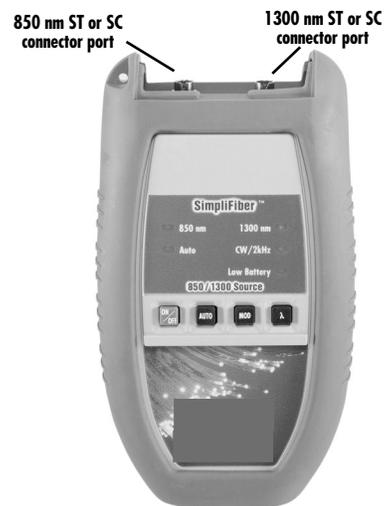
The SimpliFiber Source is an active and intelligent light source that works with the SimpliFiber Meter to verify optical cable transmission quality.
