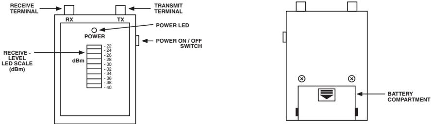
**Fig. 2-1. The Pocket Fiber Tester**
