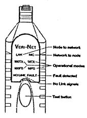
When two or more operational mode indicators are activated, the Link being tested is capable of Auto-negotiating to the highest common level of operation when a Link Partner is installed.
