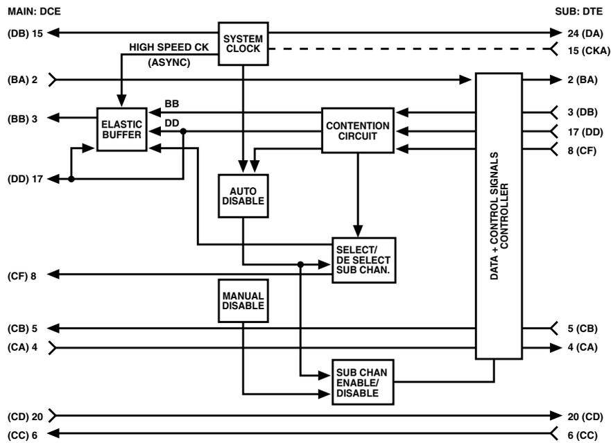
Figure A-2. Main channel DCE with sub-channel DTE.
