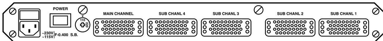
Figure 3-1. Rear panel of the V.35 Data Sharer Plus.
