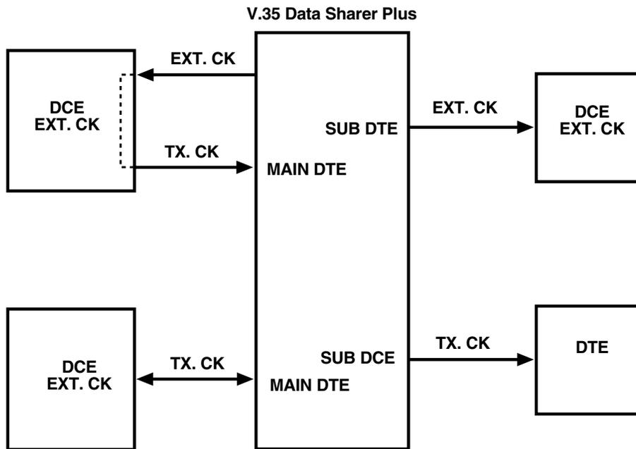
Figure 3-5. Synchronization on internal clock.
