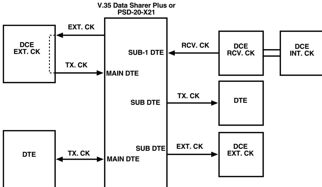
Figure 3-6. Synchronization on sub-channel 1.
