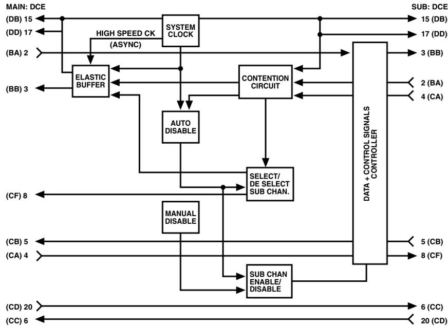
**Figure A-4. Main channel DCE with sub-channel DCE.**
