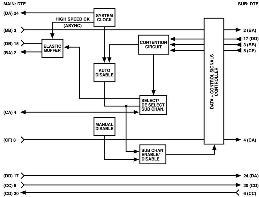
**Figure A-3. Main channel DTE with sub-channel DTE.**
