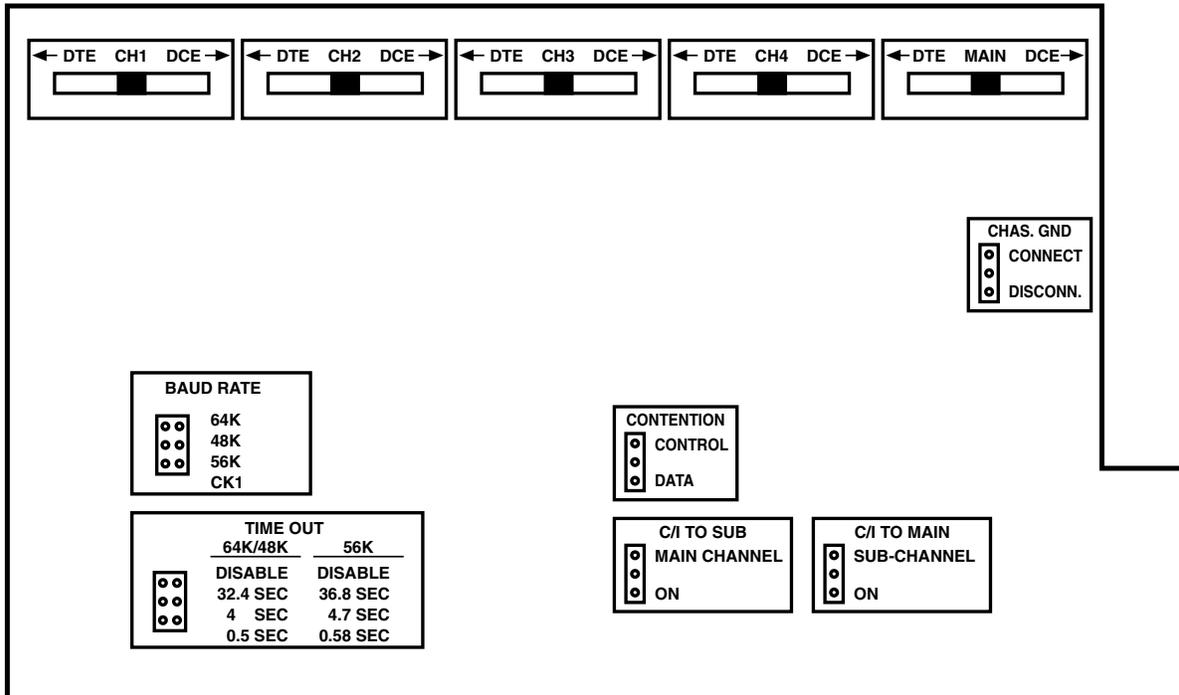
Figure 3-4. PCB layout for the PSD-20-X21.
