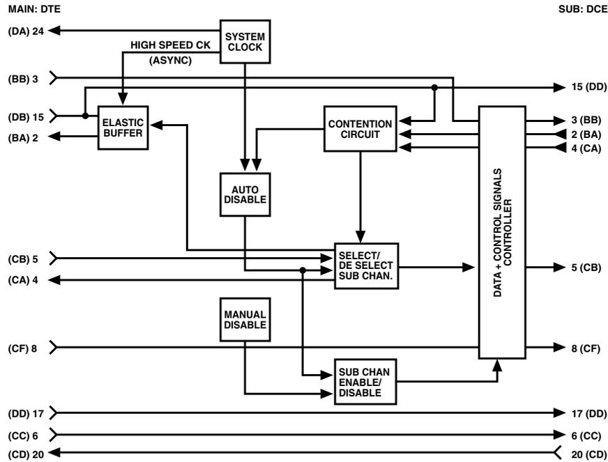
Figure A-1. Main channel DTE with sub-channel DCE.
