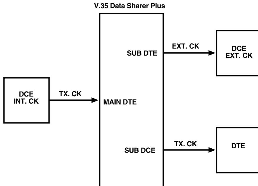
Figure 3-5. Synchronization on main-channel modem's clock.
