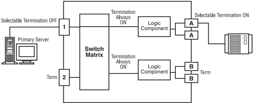
Figure 5-2. SC120A-R2 termination example 1.
