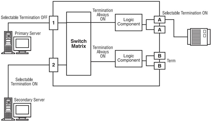
Figure 5-3. SC120A-R2 termination example 2.
