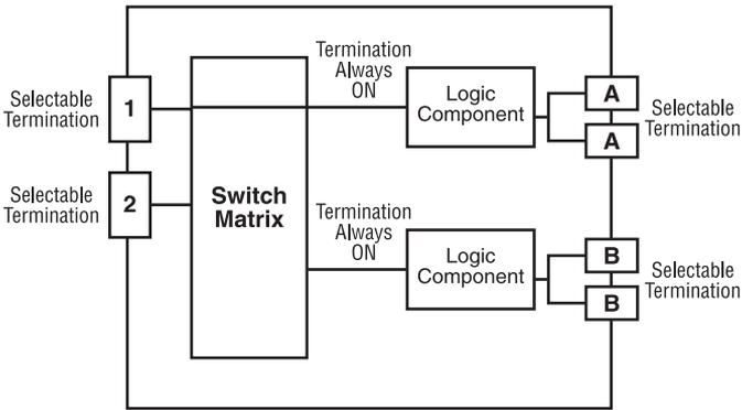
**Figure 5-1. Termination configuration.**
