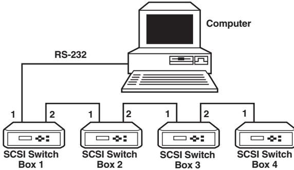
Figure 5-7. Multiple SCSI Switch configuration.
