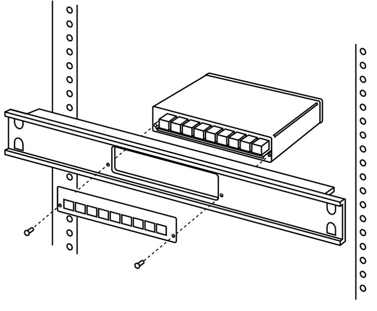
Figure 1. Rackmounting the Hub front forward.
