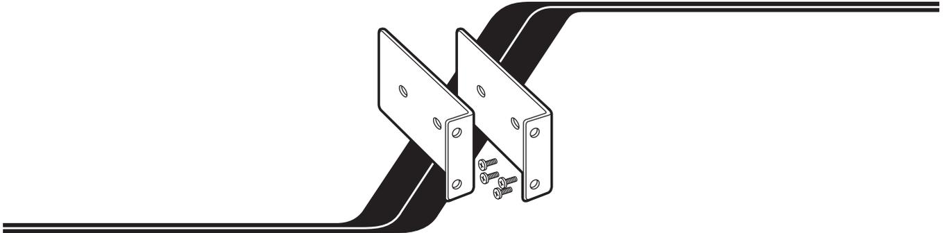
You can use your ServSwitch™ Wizard Pro Rackmount Kit to mount a ServSwitch Wizard Pro (our product code SW644A or SW648A) in a 19" rack. Each of these Kits consists of two rackmounting brackets and four screws. To use a Kit to mount a ServSwitch Wizard Pro, take these steps:
