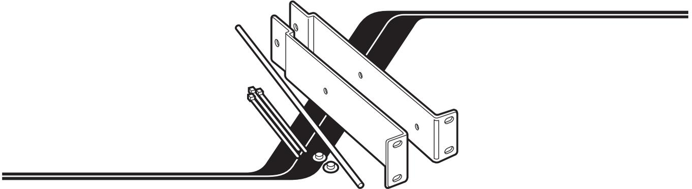
Use a ServSelect<sup>TM</sup> Rackmount Kit (our product code RMK19H) to mount a ServSelect (KV104A-R2 or KV108A-R2) in a 19" rack. Each of these Kits consists of two rackmounting side brackets, a cable-support rod, two press-on caps, and a set of tie wraps. To use a Kit to mount a ServSelect, take these steps, referring to the illustration below:
