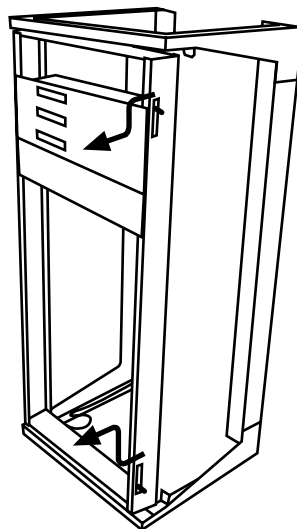
Figure 4-5. Using the levers to unlatch and open the swing frame.
