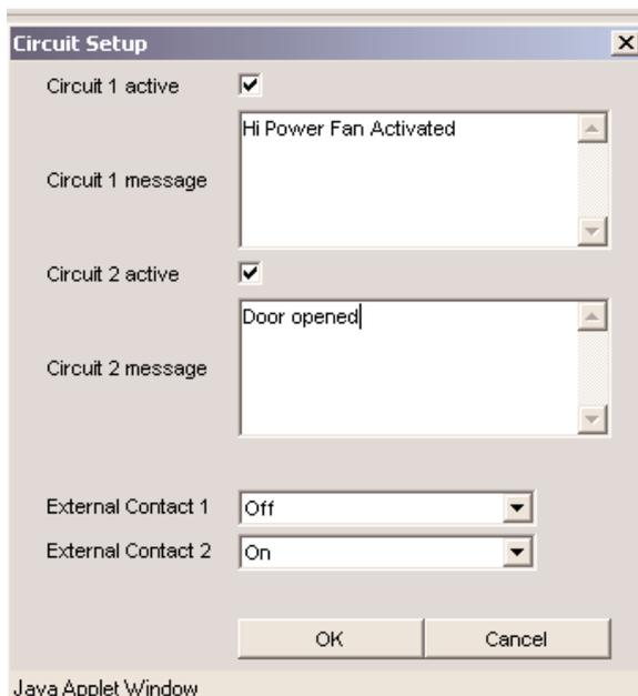
**Figure 6-11. Web interface external circuit setup.**
