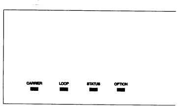
(this assumes that no option is fitted and the unit has been installed correctly). The front panel LEDs show general status of operation as shown here. These LEDs have two colours to identify various states. The normal operating condition is shown in **bold** in the table below, and coloured **Green** on the front panel. If the light is **red** a fault has been detected.
