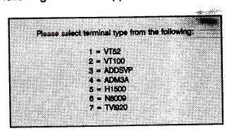
The terminal type or emulation in use should be selected by pressing the relevant number key on the PC or terminal. The monitor will now show the basic configuration screen for the multiplexer setup. This is formatted as below:
