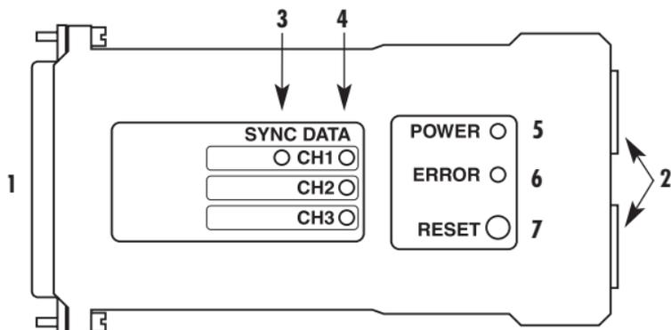
Figure 4-1. The X.25 PAD-2's top panel, showing the external indicators, connectors, and reset button.
