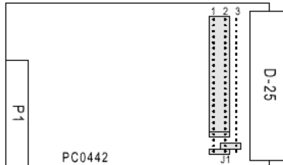
Figure A-7. DTE, V.35 and RS-530
