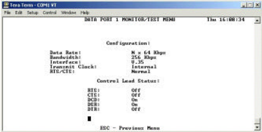
Figure 4-10. A Data-Port Monitor/Test screen (Data Port 1 shown).
