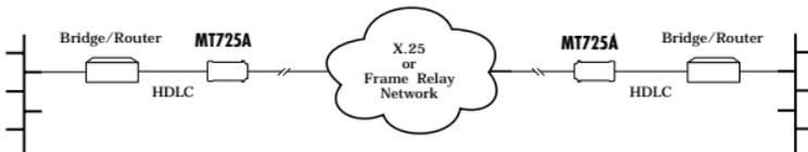
**Figure 2-1. Fradswitch-2 A/S connecting bridge/routers over X.25/Frame Relay.**
