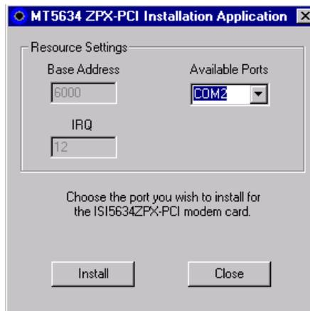
7. An available COM port is assigned to the modem. You may change the COM port assignment by either typing in or selecting an unused COM port from the list. Remember, or write down the COM port number for the modem; you'll need to know it later when you install the modem to that port.
