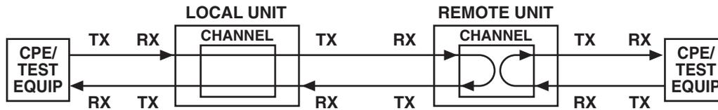
**Figure 5-4. Remote Channel Loopback Diagram.**
