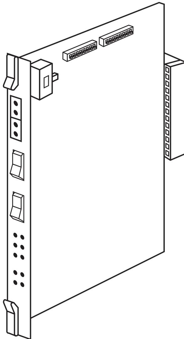
Figure 2-1. T1 CSU/DSU Card.
