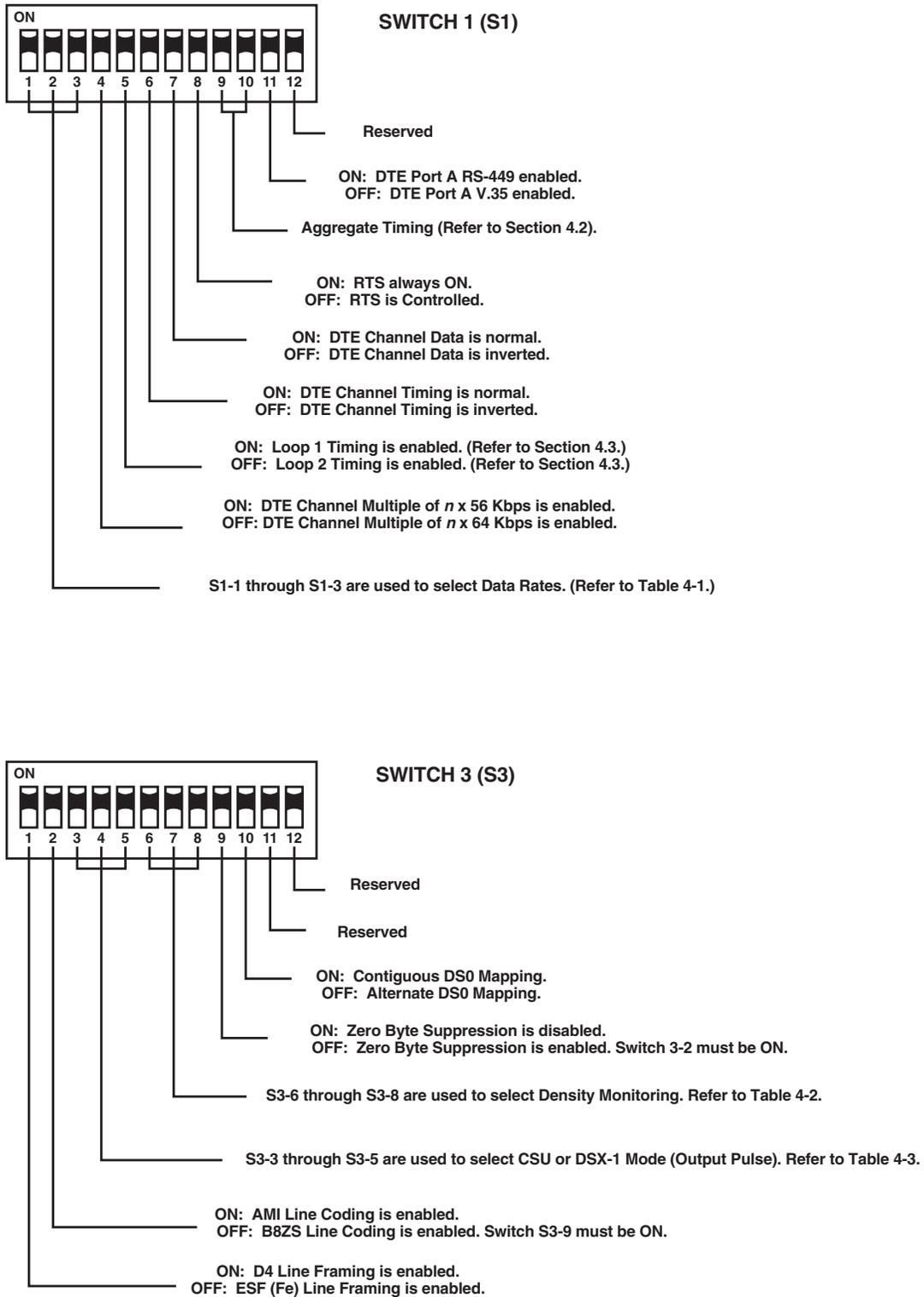
Figure 4-1. Configuration DIP Switches.
