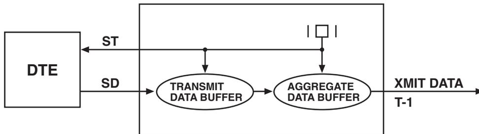
Figure 4-2. Internal (Master) Crystal Timing Diagram.
