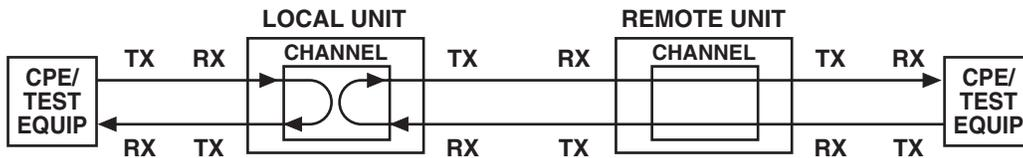
**Figure 5-3. Local Channel Loopback Diagram.**
