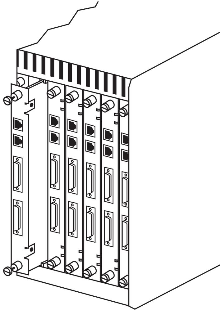
Figure 3-2. Installing the I/O Interface Module.
