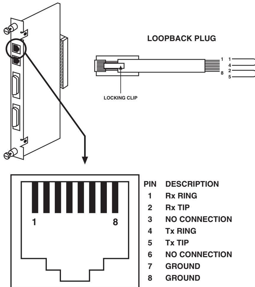
Figure 2-4. NET Interface Pinout.
