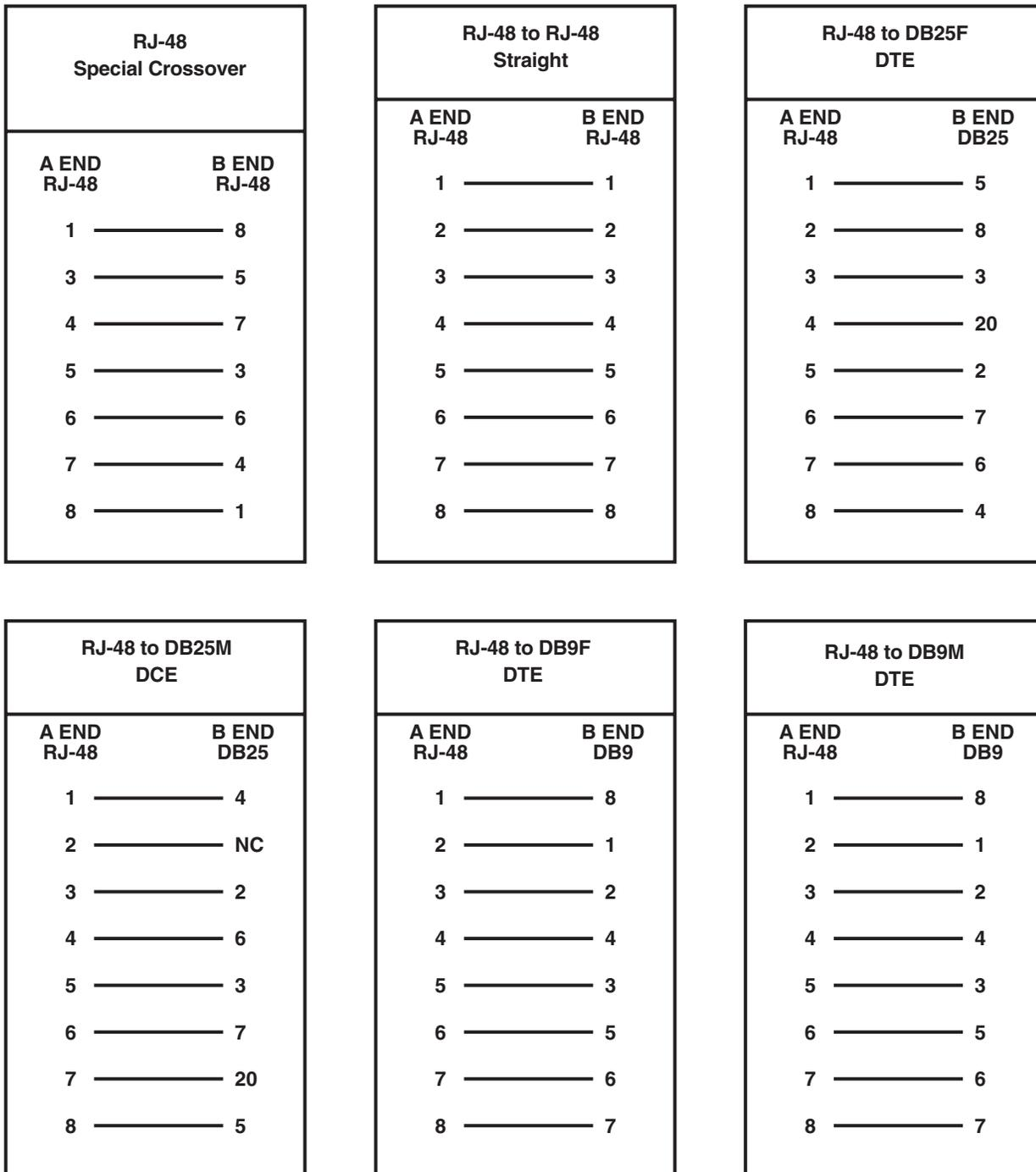
Figure C-1. Common Cable Pinouts (continued).
