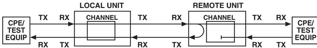
**Figure 5-2. Remote Aggregate Loopback Diagram.**
