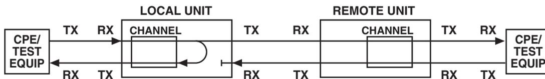
Figure 5-1. Local Aggregate Loopback Diagram.
