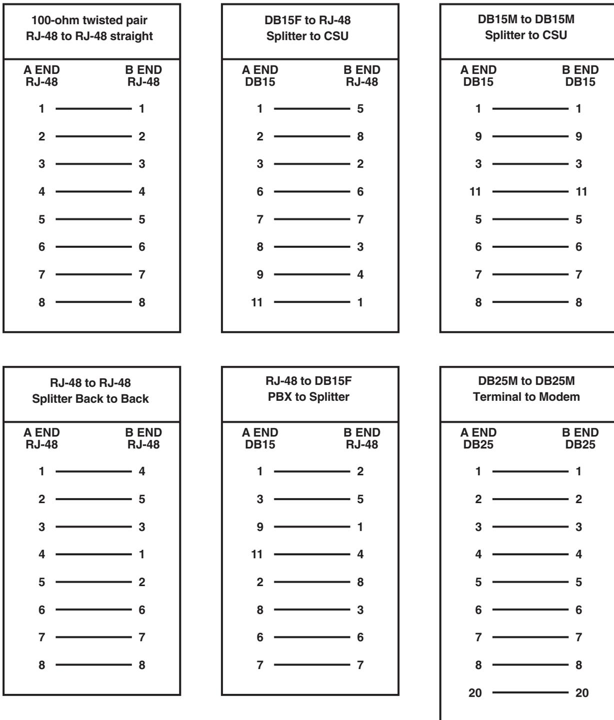
Figure C-1. Common Cable Pinouts.
