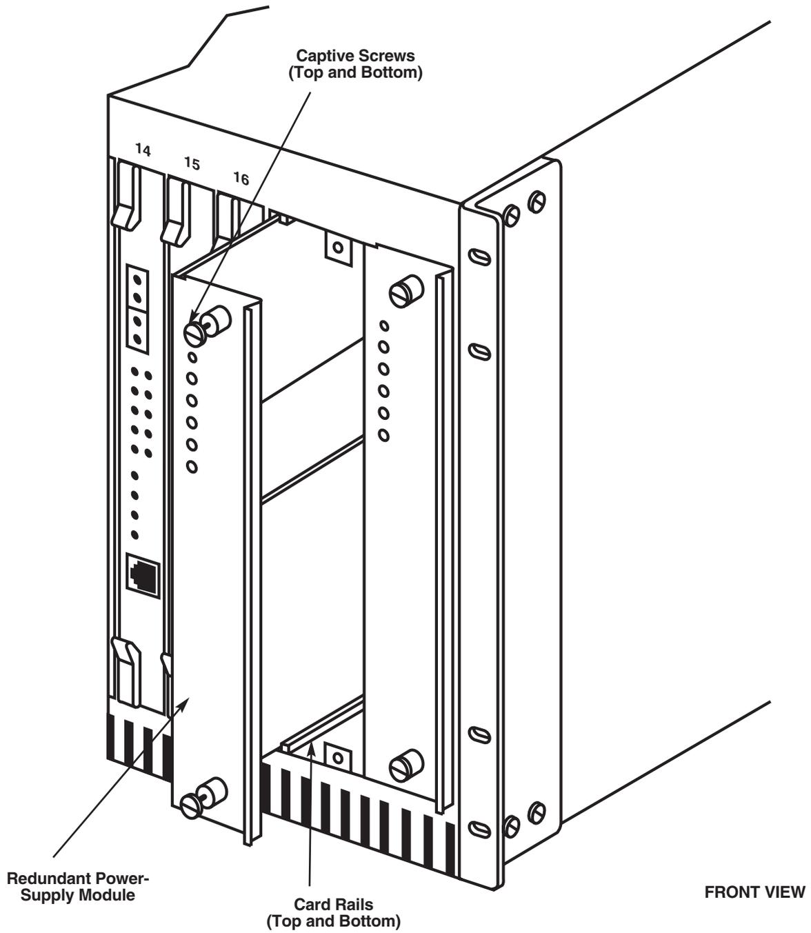
**Figure 3-11. Installing the Power-Supply Module.**
