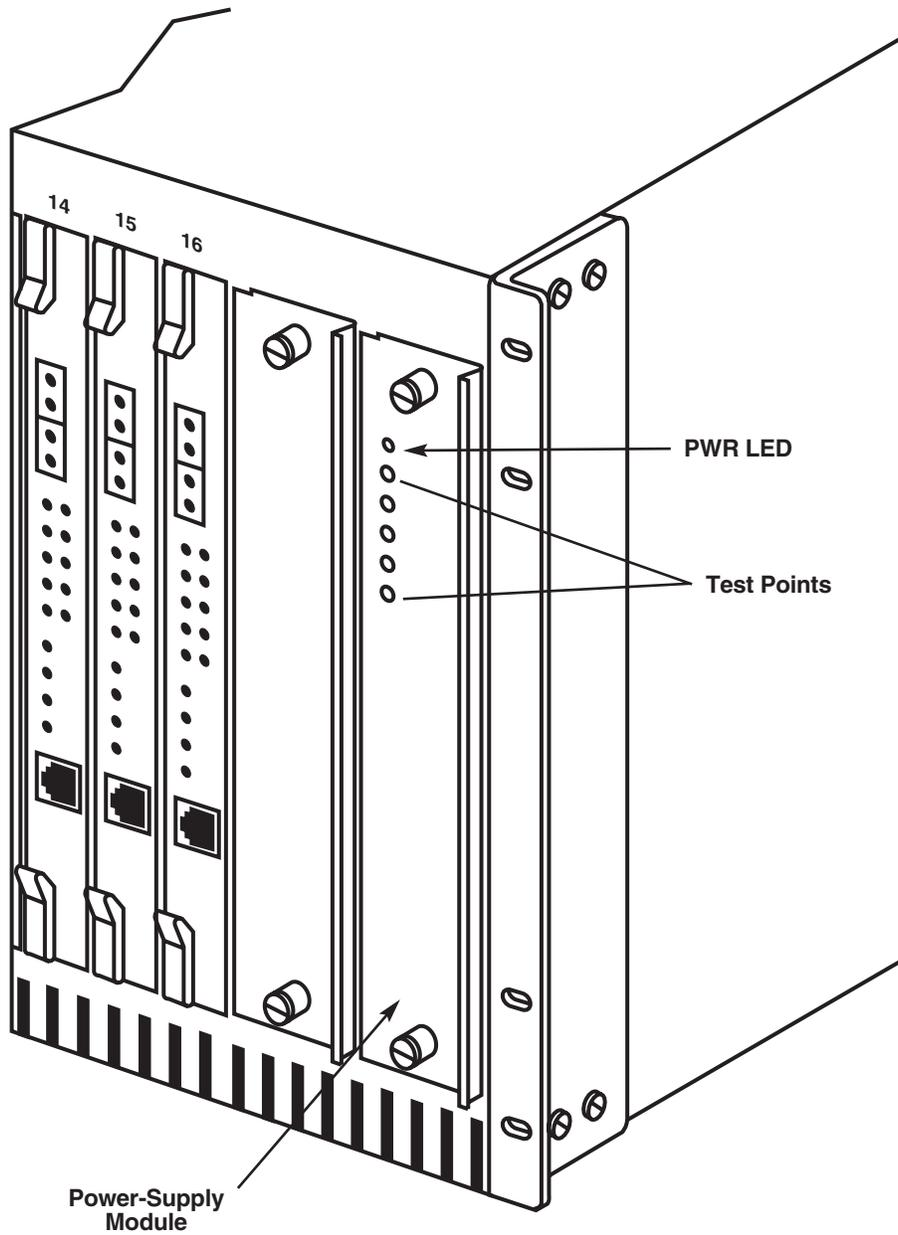
Figure 4-2. Power-Supply Module (Front View).
