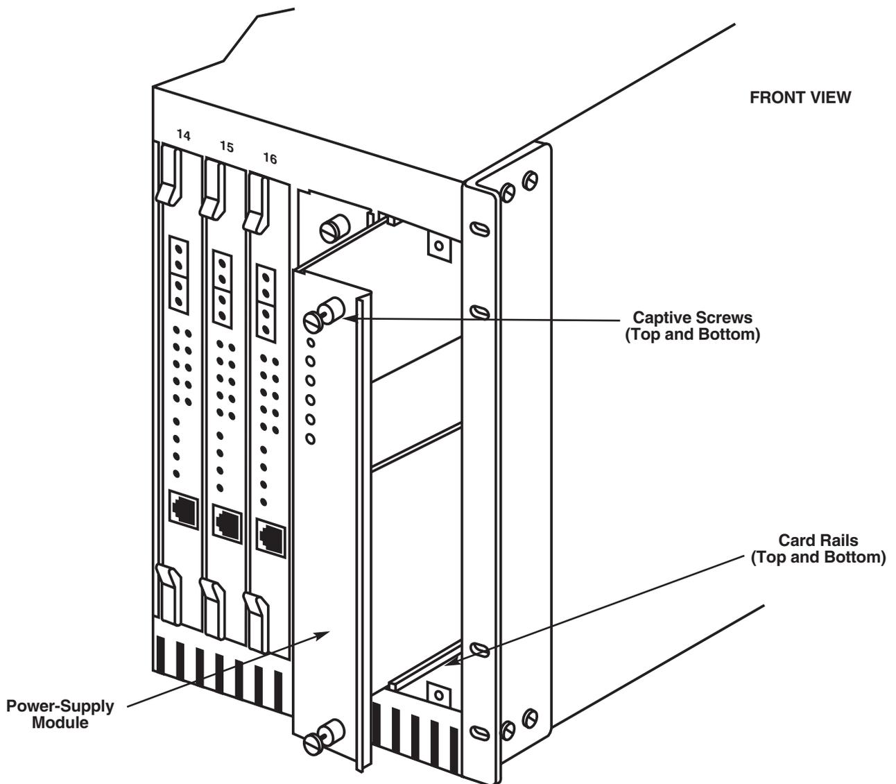
Figure 4-4. Reseating a Power-Supply Module.
