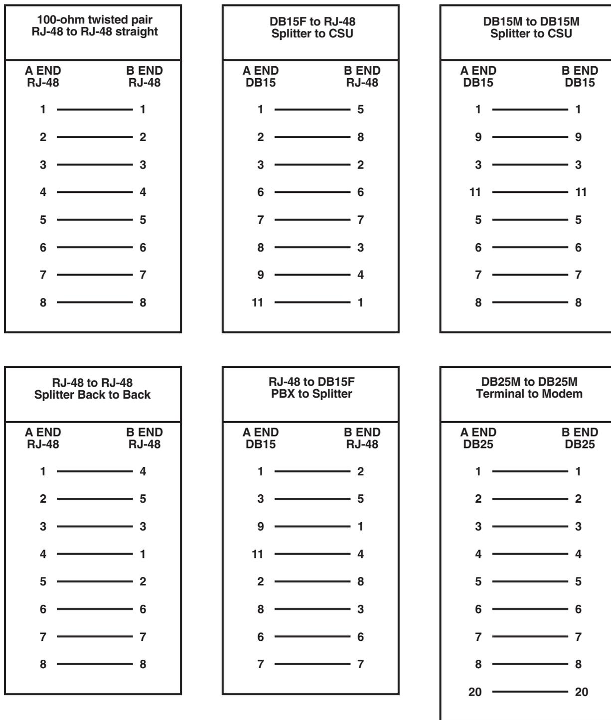
Figure 3-9. Common Cable Pinouts.
