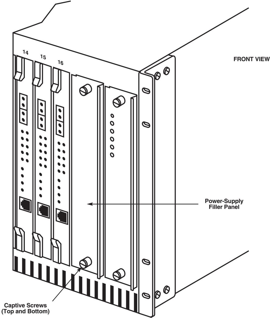
Figure 3-10. Removing the Filler Panel.
