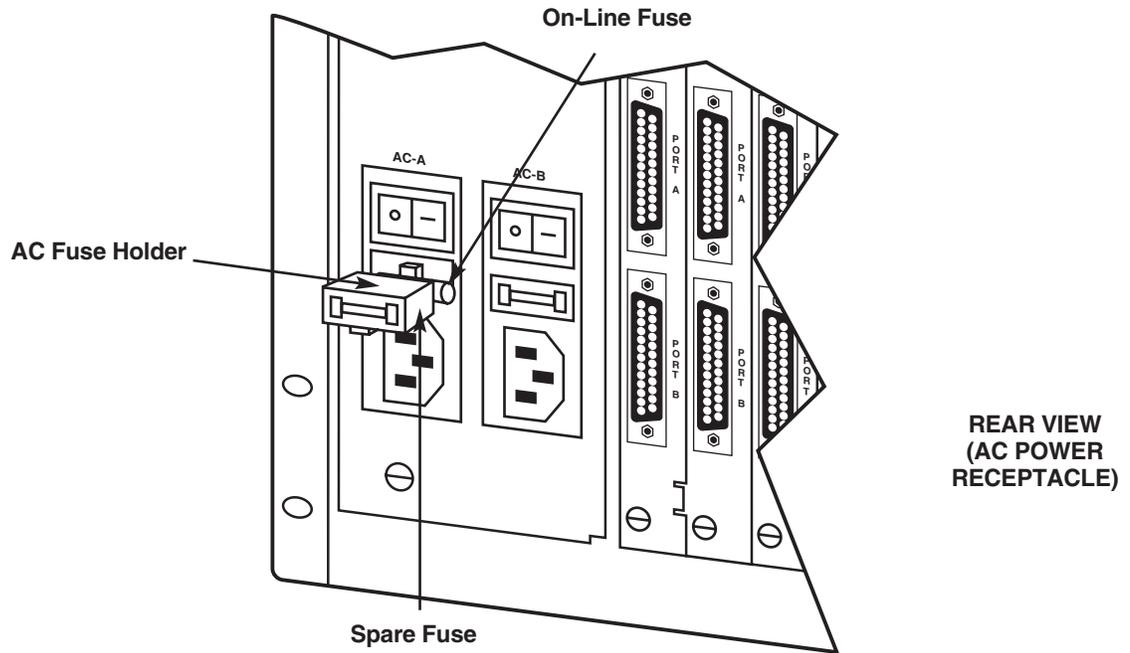
**Figure 4-5. Checking/Replacing an AC Fuse.**
