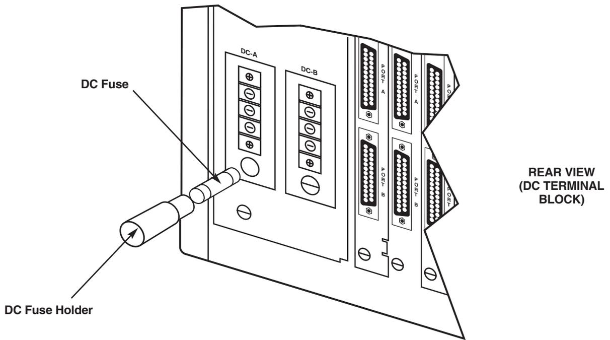
**Figure 4-6. Checking/Replacing a DC Fuse.**
