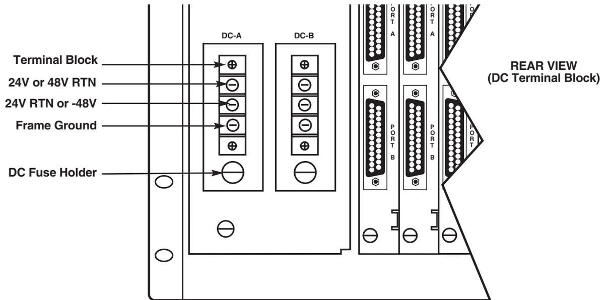
Figure 4-3. AC Receptable and DC Terminal Block.
