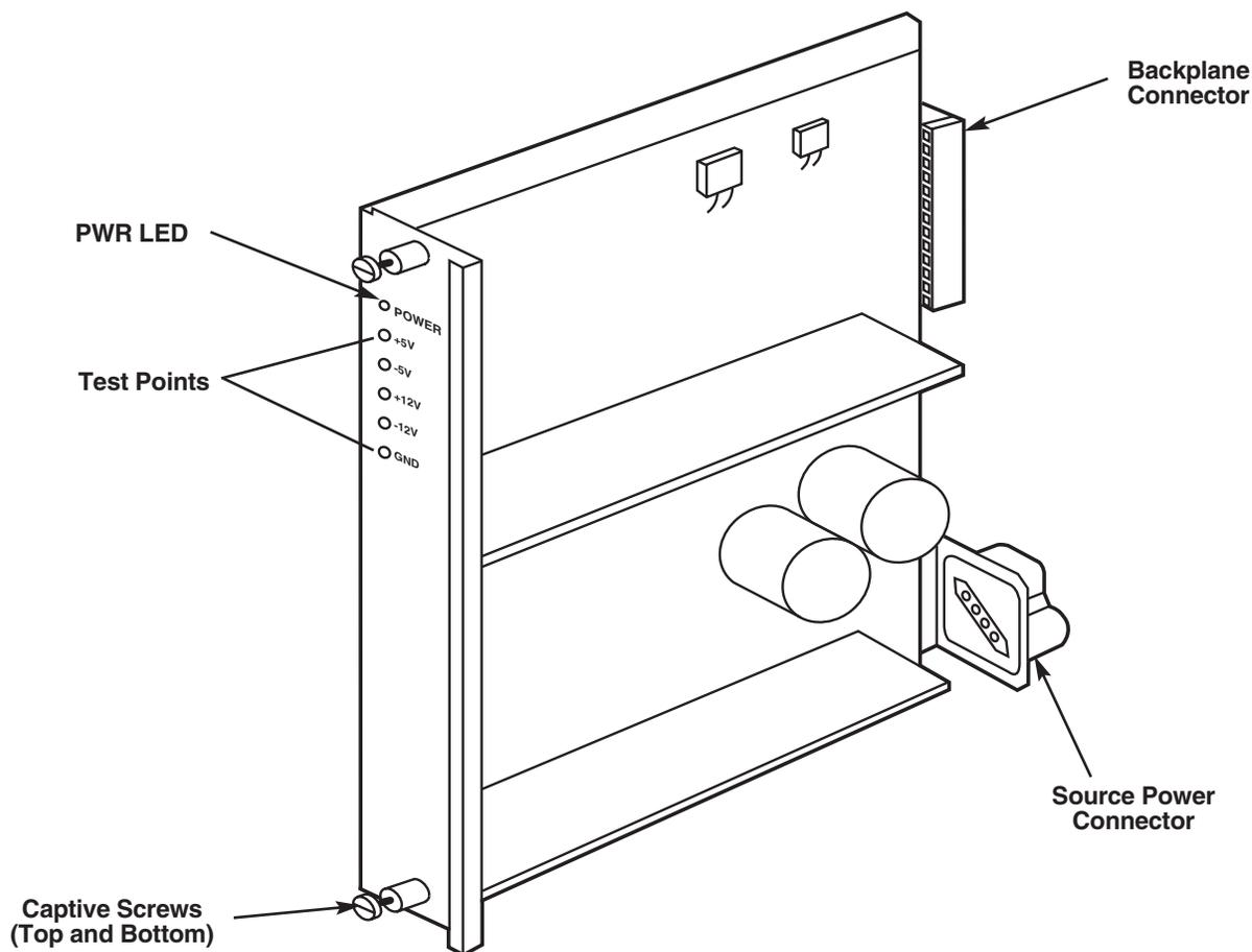
Figure 2-5. Power-Supply Module.
