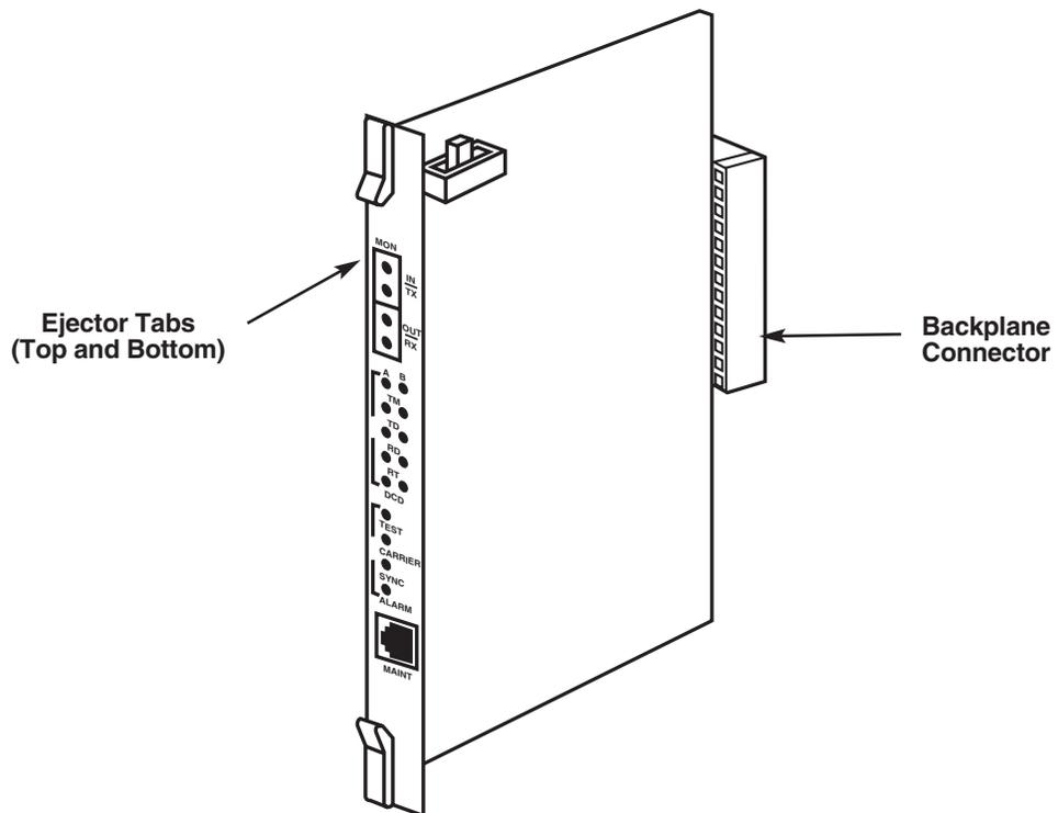
Figure 2-6. FT1 Mux Card-2D (MT520A).
