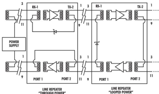
Figure 3-2. Telco Simplex Power Arrangement.
