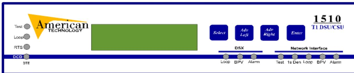
**Figure 2-1 1510 T1/FT1 CSU/DSU Front Panel View**
