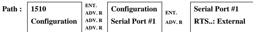
The control lead RTS (Request To Send) may be set to either External or Constant. An External setting follows the DTE equipment RTS setting where as a Constant setting ignores the DTE and assumes RTS is present at all times. Press the ENTER key until the desired selection is displayed. The selected option appears on the bottom line of the LCD.
