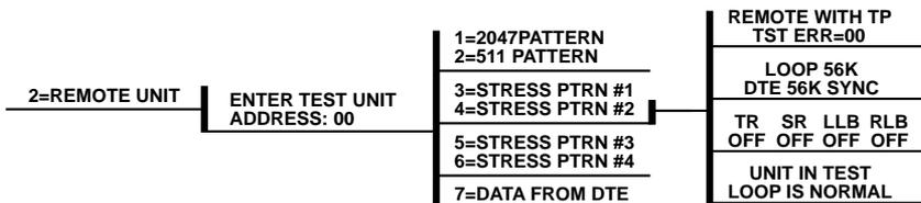
Fig. 4-27. Remote Unit Submenu of 2=Test.
