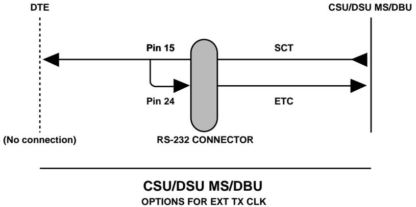
**Fig. B-2. EIA 232 Connector for 56 Kbps Application.**
