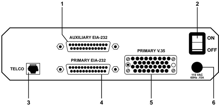
**Fig. 2-2. CSU/DSU MS Rear View.**
