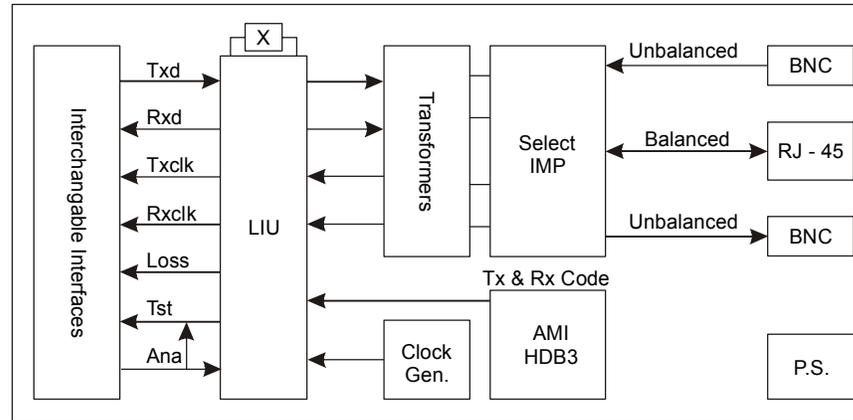
Figure 1-2. Block Diagram, E1 Converter
