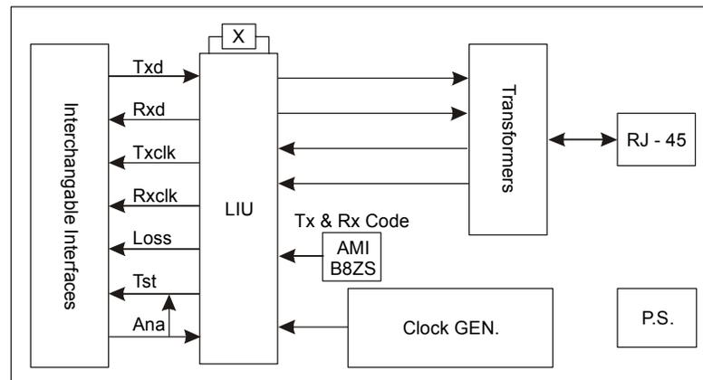
Figure 1-3. Block Diagram, T1 Converter
