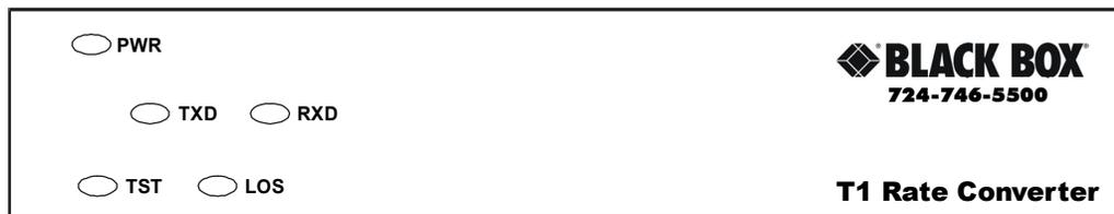
*Figure 3-2. T1 Converter Front Panel*
