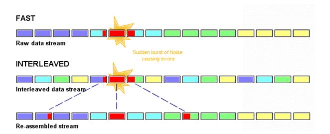
If your line is particularly susceptible to bursts of noise then interleaving should improve your VDSL experience. Noise on the line caused by crosstalk will not damage a complete block of data, but parts of data blocks, which can be re-assembled by CRC.
