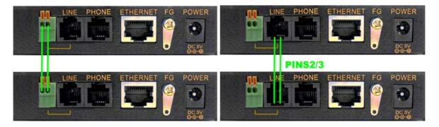
The RJ-11 Phone port of the Transmitter can be connected to a PBX (ab) or your incoming 2-wire ISDN connection. The RJ-11 Phone port of the Receiver can be connected to an analogue telephone, an analogue Modem or your NTBA.
