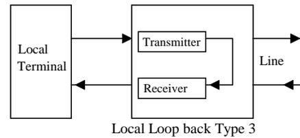
Local modem is disconnected from the line. Transmit line is looped to receive line on local modem. Data transmitted by the terminal are sending back by the local modem. This loop back permits to test only the local modem.
