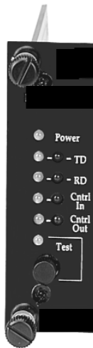
Figure 5-1. Front Panel, Showing LED Positions.
