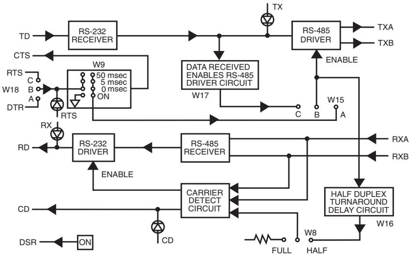
**Figure 3-2. Simplified Functional Block Diagram (DCE Operation).**
