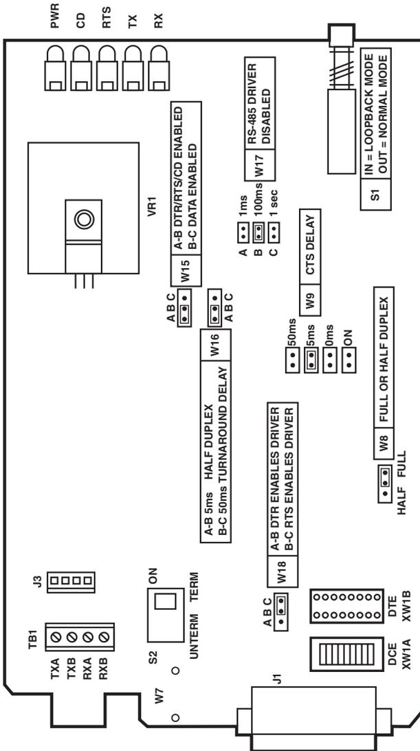
Figure 3-1. PCB Layout.
