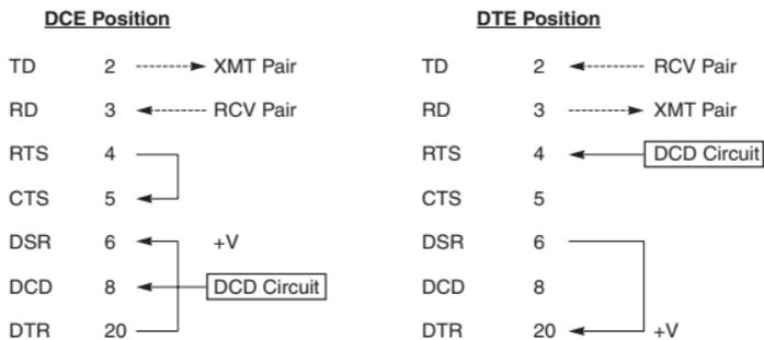
**Figure 3-3. DCE/DTE Switch Configuration.**
