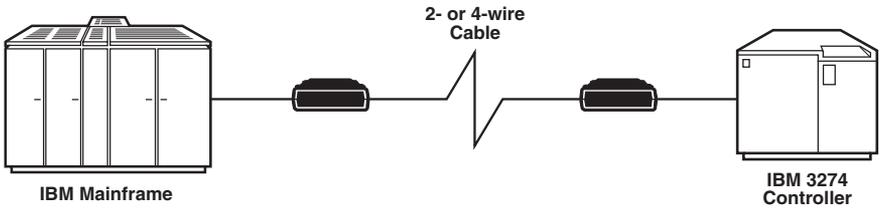
**Figure 2-1. Point-To-Point Synchronous Application.**
