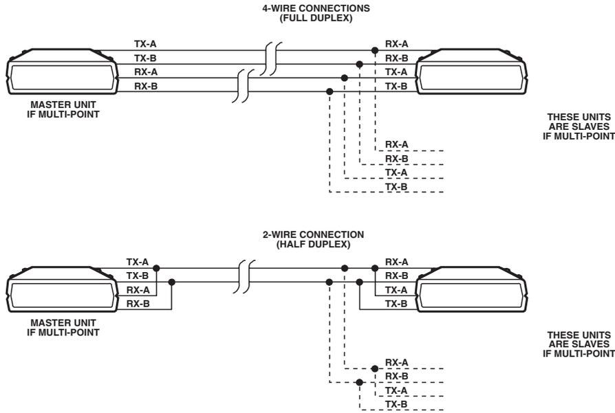
Figure 3-1. Inter-Connect Wiring Diagram.
