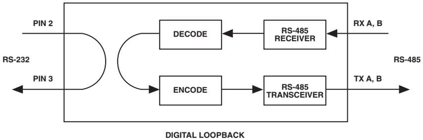
**Figure 5-2. Digital Loopback Test.**
