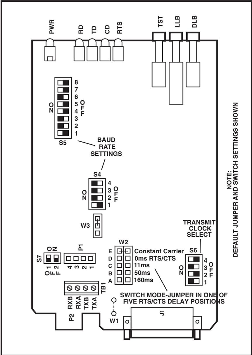
Figure 3-2. Printed Circuit Board Layout.
