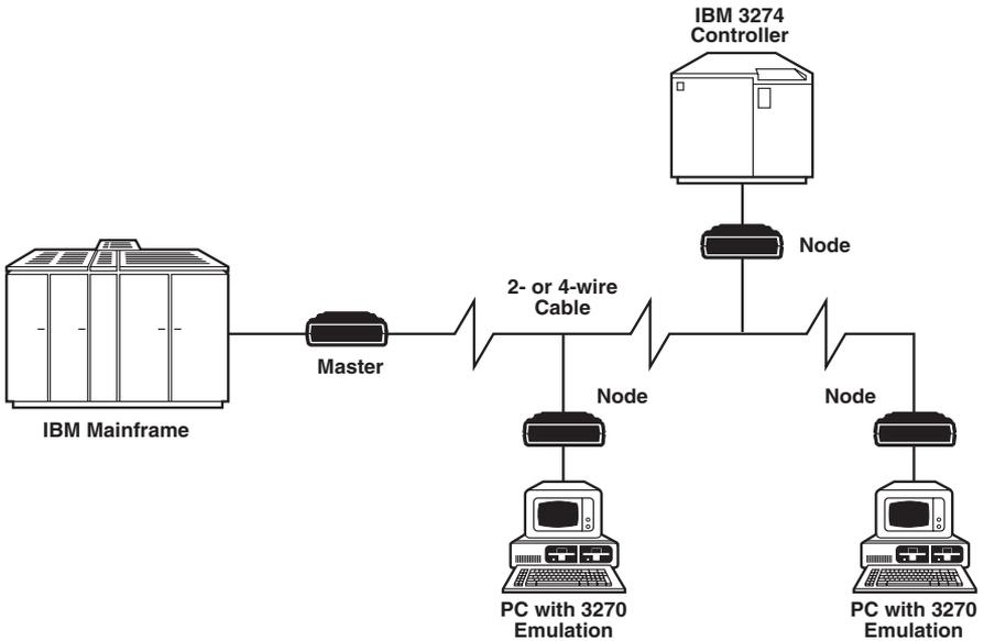
**Figure 2-2. Multipoint Synchronous Application.**
