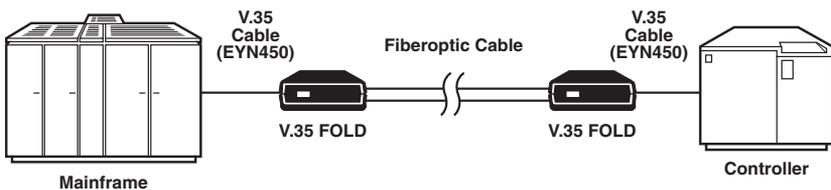
Figure 1. The V.35 FOLD is designed for a point-to-point application.
