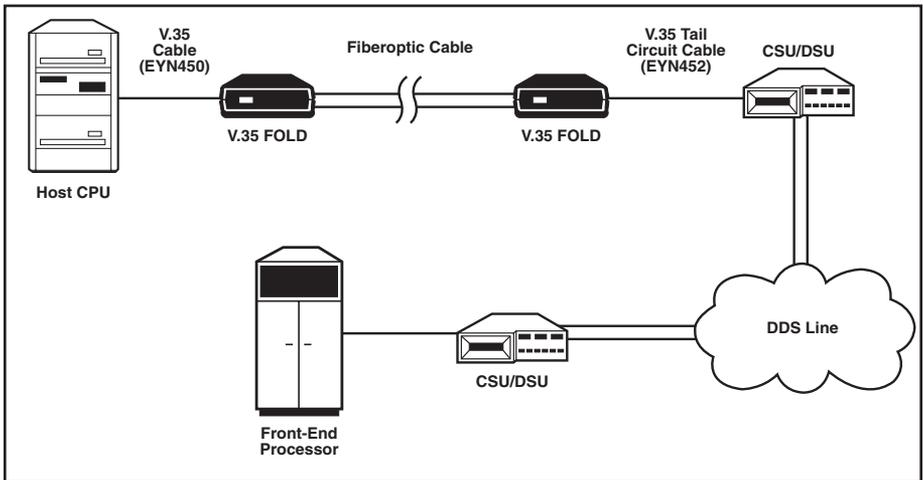
Figure 7. V.35 FOLD tail-circuit application.
