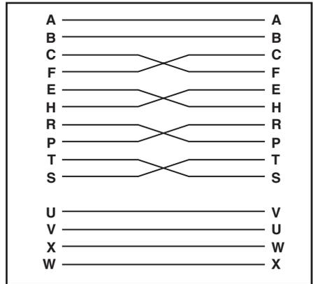
Figure 6. Cable pinouts for V.35 tail circuit applications.
