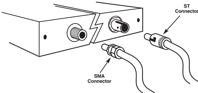
Figure 5. Fiber Optic Connectors
