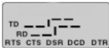
Figure 1: The DataSpy™ LCD display.
