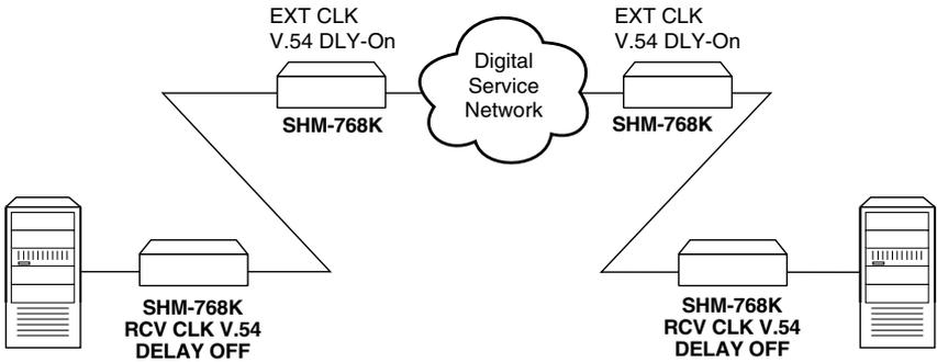
**Figure 2-2. Tail-end for DDS Service Application.**
