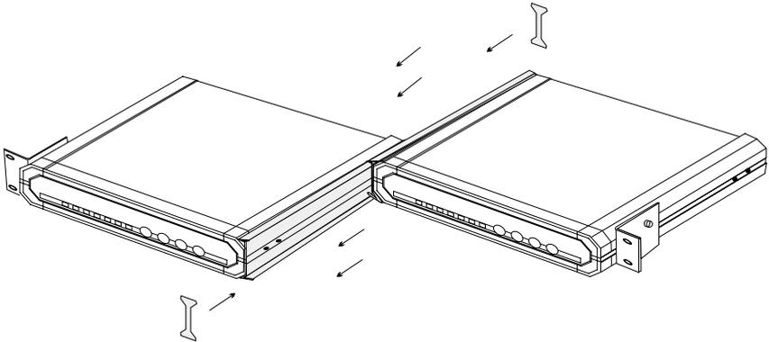
**Figure B-3. Installation of Two Units, Part 2.**
