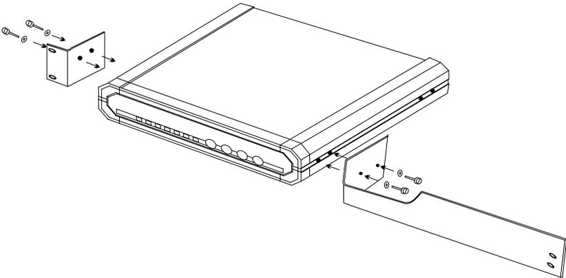
Figure B-1. Installation of a Single Unit.
