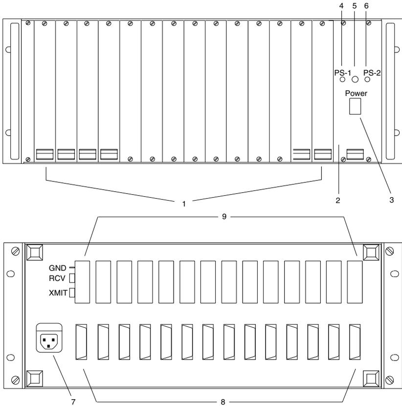
**Figure 6-2. Rack Enclosure with Dual Power Supply.**
