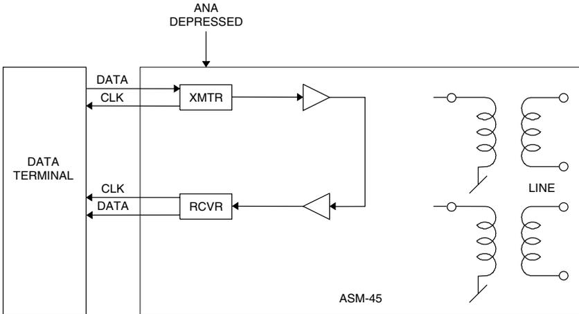
**Figure 5-3. Local SHM-768K in Analog Loopback.**
