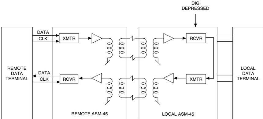
**Figure 5-5. Local SHM-768K in Digital Loopback.**
