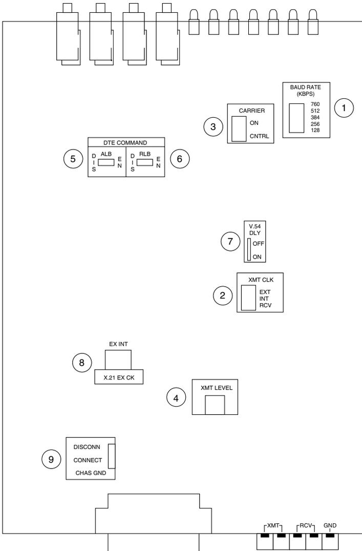
Figure 3-2. Printed Circuit Board Layout.
