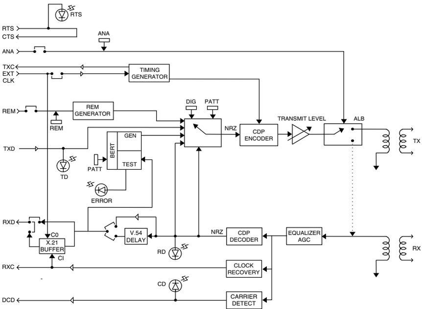
Figure 2-3. SHM-768K Block Diagram.
