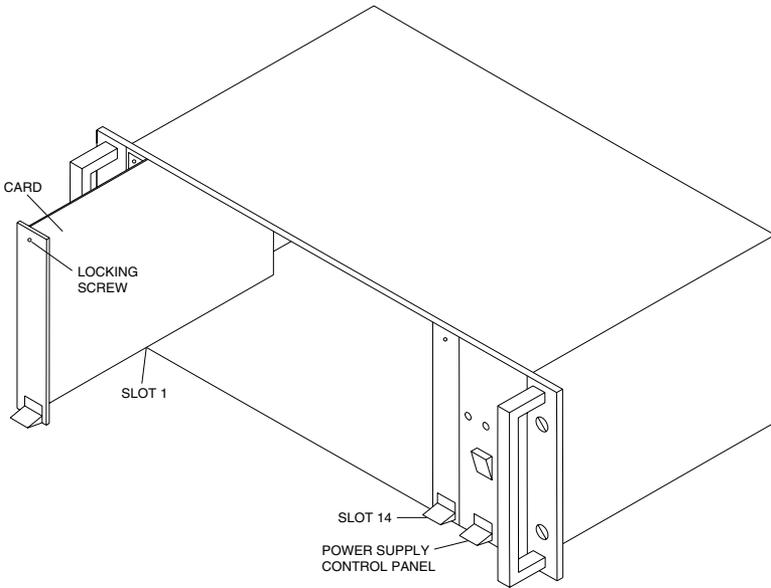
**Figure 6-1. Rack Installation.**
