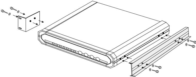
**Figure B-2. Installation of Two Units, Part 1.**
