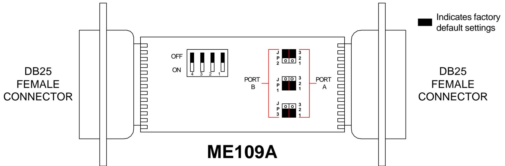
The V.35 Sync Modem Eliminator is equipped with one internal four position DIP switch and Six internal jumpers that allow configuration for a wide range of applications. All switches and jumpers are located on the inside of the unit. The DIP switch is located on the daughter board and the jumpers are located on the main PC Board.
