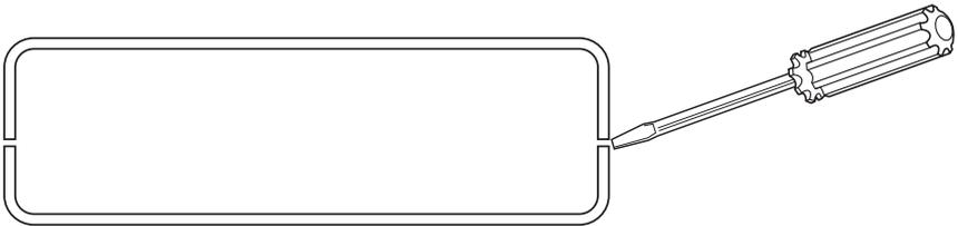
**Figure 4-5. Opening the case with a small screwdriver.**
