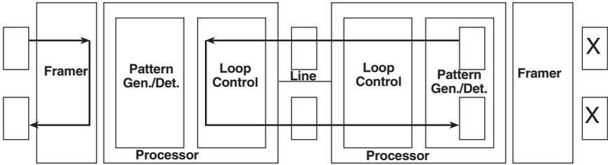
Figure 5-6. Local loop mode 2 with 511/511E.
