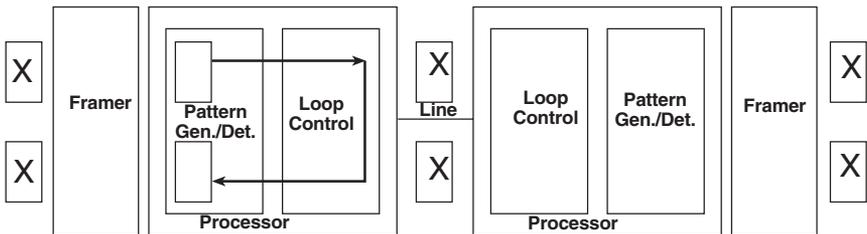
**Figure 5-5. Local loop mode 1 with 511/511E.**
