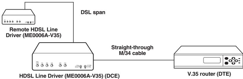
**Figure 4-2. Connecting the Line Driver to a V.35 serial DTE.**
