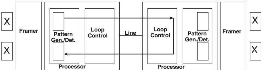
**Figure 5-8. Remote loop with 511/511E.**
