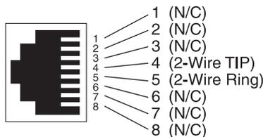
**Figure 4-1. RJ-45 twisted-pair line interface.**
