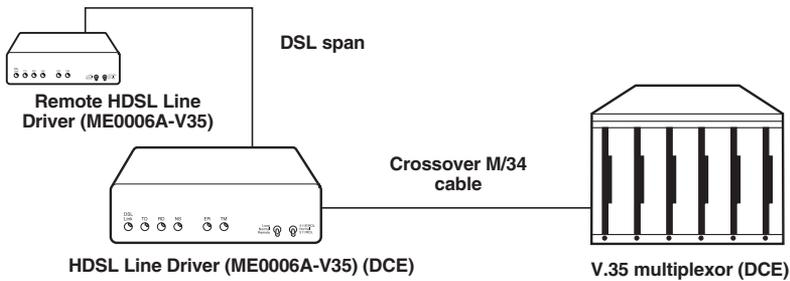
Figure 4-3. Connecting the Line Driver to a V.35 serial DCE.
