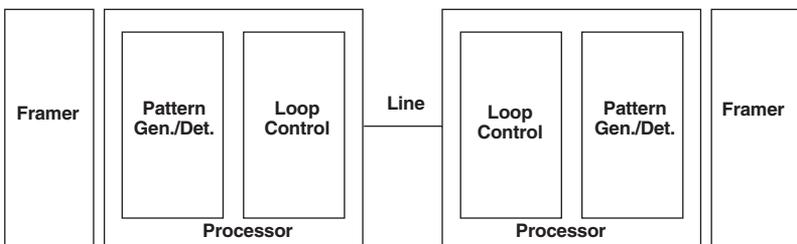
**Figure 5-2. The major elements used in loopback and pattern tests in the Line Driver.**
