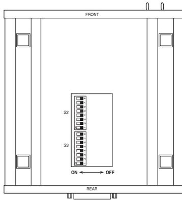
**Figure 3-1. Underside of the HDSL Line Driver, showing the location of the DIP switches.**
