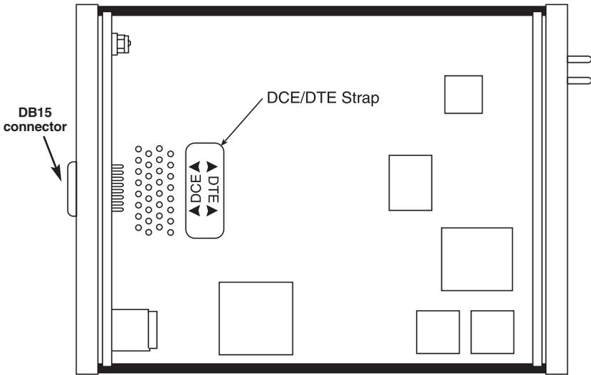
Figure 4-6. Setting the DCE/DTE strap.
