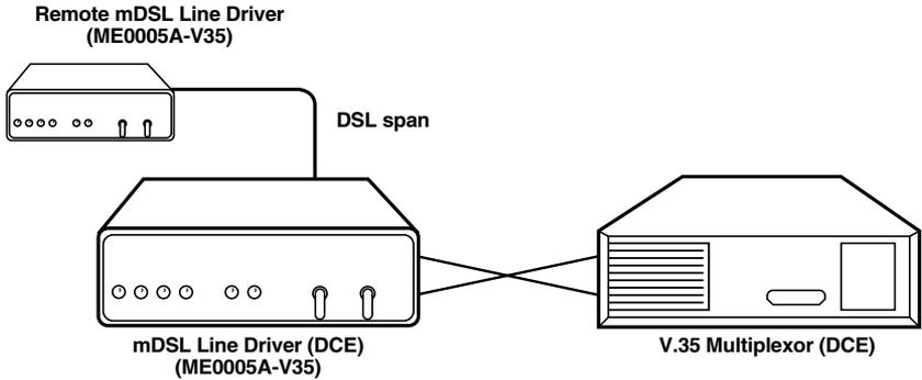
Figure 4-3. Connecting the Line Driver to a V.35 serial DCE.
