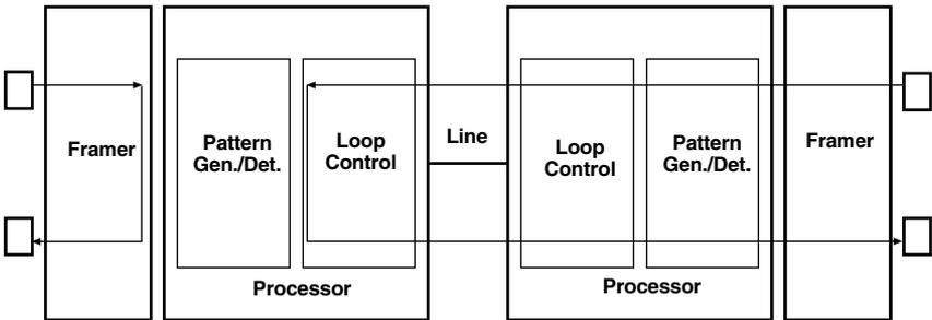
**Figure 5-4. Block diagram local loop mode 2.**
