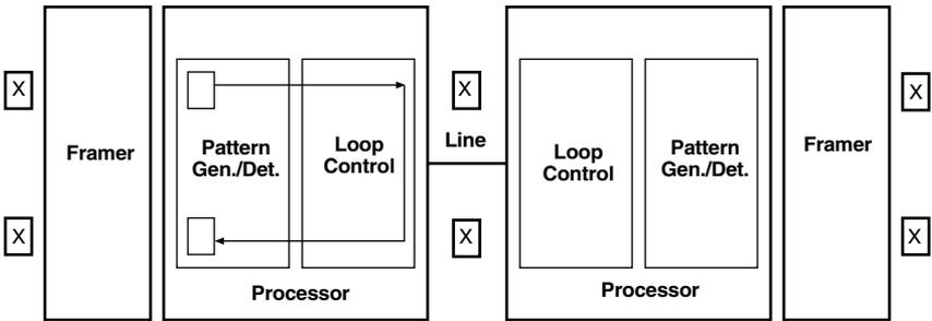
**Figure 5-5. Block diagram local loop mode 1 with 511/511E.**
