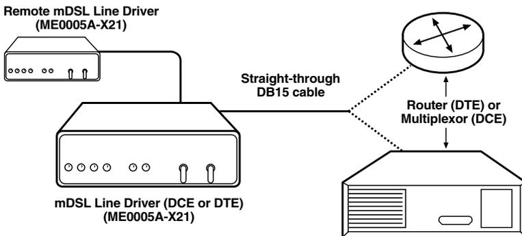
Figure 4-4. Connecting the Line Driver to a X.21 DTE or DCE.
