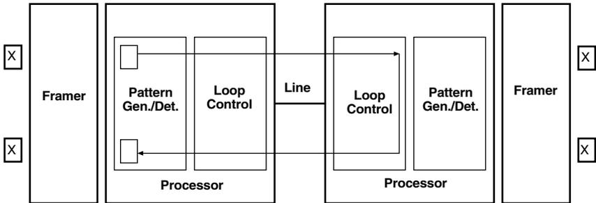
**Figure 5-8. Block diagram remote loop with 511/511E.**
