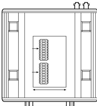
**Figure 3-1. Underside of the mDSL Line Driver, showing the location of the DIP switches.**
