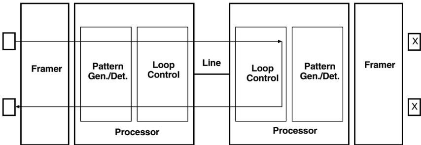
Figure 5-7. Block diagram remote loop.
