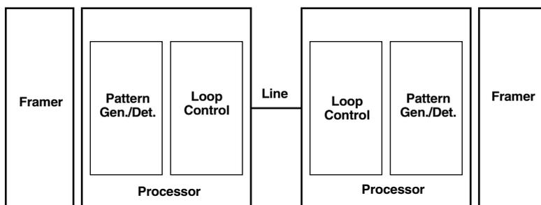
**Figure 5-2. Block diagram: two mDSL Line Drivers communicating over the DSL span.**
