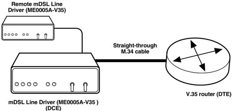
**Figure 4-2. Connecting the Line Driver to a V.35 serial DTE.**
