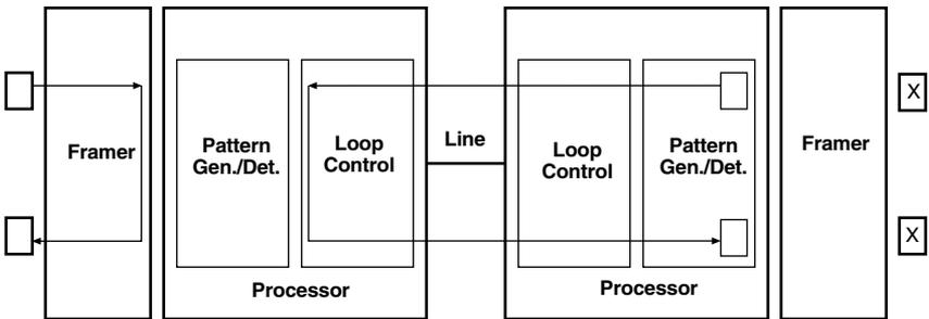
**Figure 5-6. Block diagram local loop mode 2 with 511/511E.**
