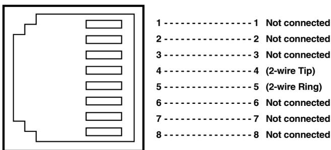
**Figure 4-1. RJ-45 twisted-pair line interface.**
