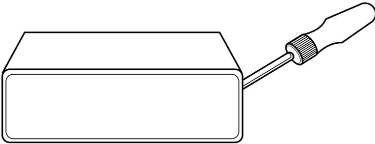
**Figure 4-5. Opening the case with a small screwdriver.**
