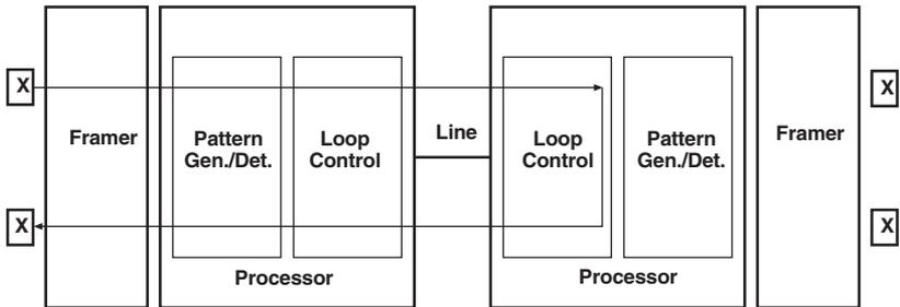
**Figure 5-8. Remote loop with 511/511E.**
