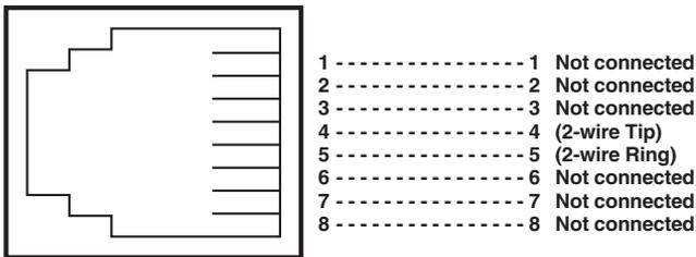
Figure 4-5. Twisted-pair line interface.
