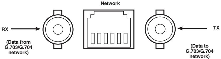
Figure 4-4. 75-ohm dual coaxial G.703 interface.
