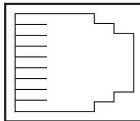
**Figure 4-3. 120-ohm RJ-48C G.703 interface.**
