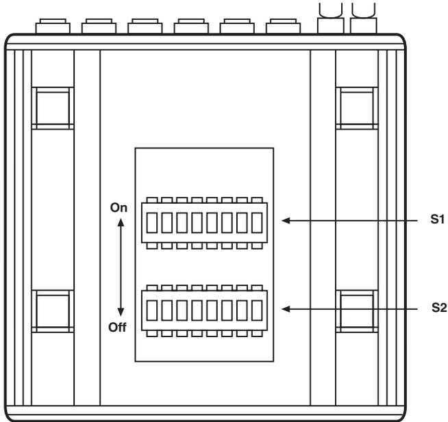
**Figure 3-1. Underside of the mDSL Line Driver, showing the location of the DIP switches.**
