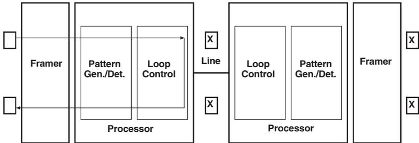
**Figure 5-5. Local loop mode 1 with 511/511E.**
