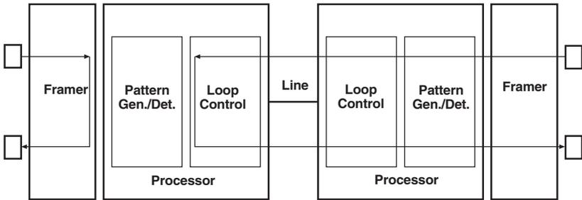
Figure 5-6. Local loop mode 2 with 511/511E.
