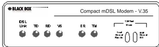
Figure 10. Compact mDSL Modem Front Panel
