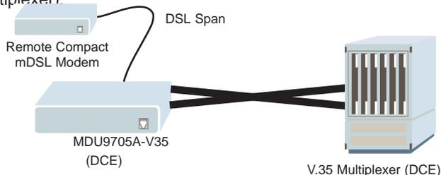
Figure 5. Connecting the MDU9705A-V35 to V.35 Serial DCE
