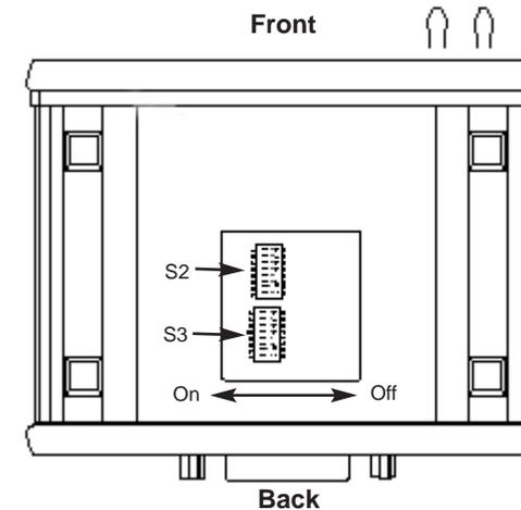
Figure 1. Underside of Compact mDSL Modem, Showing Location of DIP Switches
