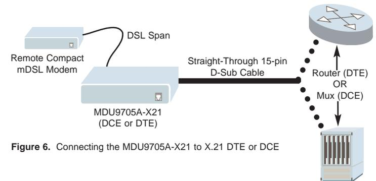
Figure 6. Connecting the MDU9705A-X21 to X.21 DTE or DCE
