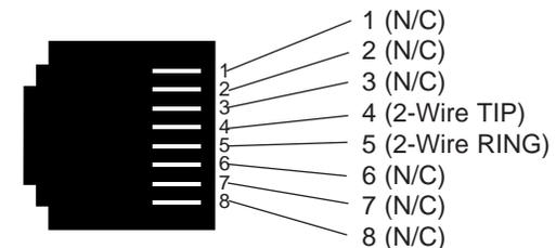
Figure 4. Compact mDSL Modem RJ-45 twisted pair line interface.
