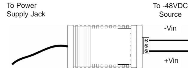
Figure 9. Connecting DC Power to the 48VDC Power Supply.
