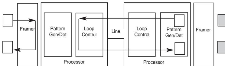
Figure 15. Block Diagram Local Loop Mode 2 with 511/511E
