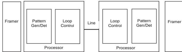
Figure 11: Block Diagram Compact mDSL Modem
