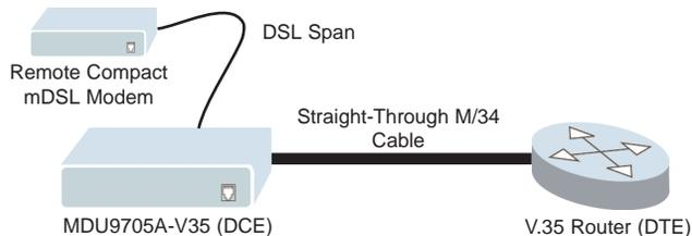
Figure 4. Connecting the MDU9705A-V35 to V.35 Serial DTE
