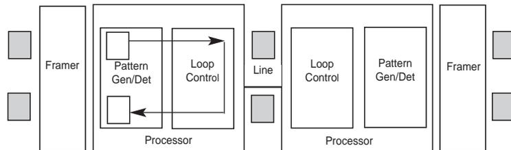
Figure 14. Block Diagram Local Loop Mode 1 with 511/511E
