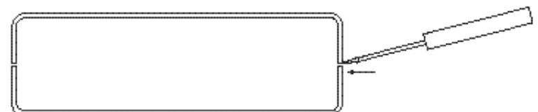
Figure 7. Opening the case with a small screwdriver
