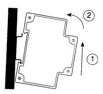
De-mounting a modem module Lift the module (1) and twist it out from the top (2) and the module is released from the DIN rail.
