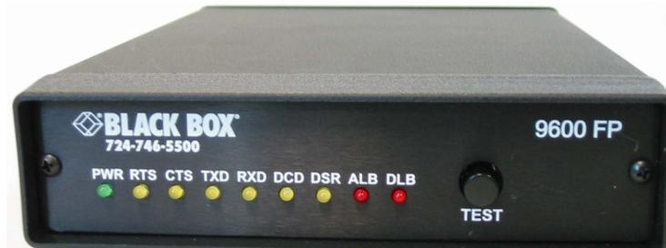
**Figure 2-2. Front View of the Modems**
