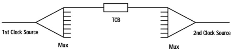
**Figure 4-1. Connecting sub-channels of two multiplexers operating with different clocks.**
