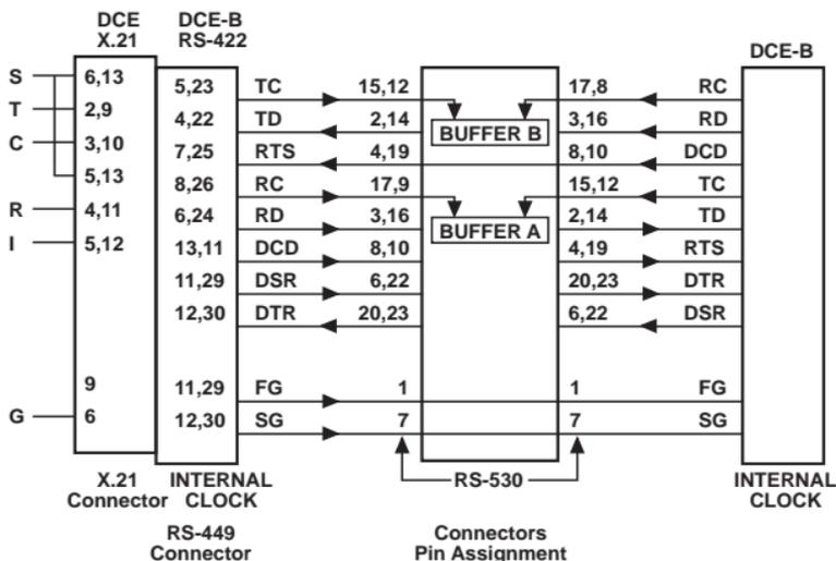
Figure 3-1. Schematic Diagram of Data Flow through the TCB.
