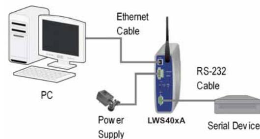
Figure 6. Wired Connection for Configuration
