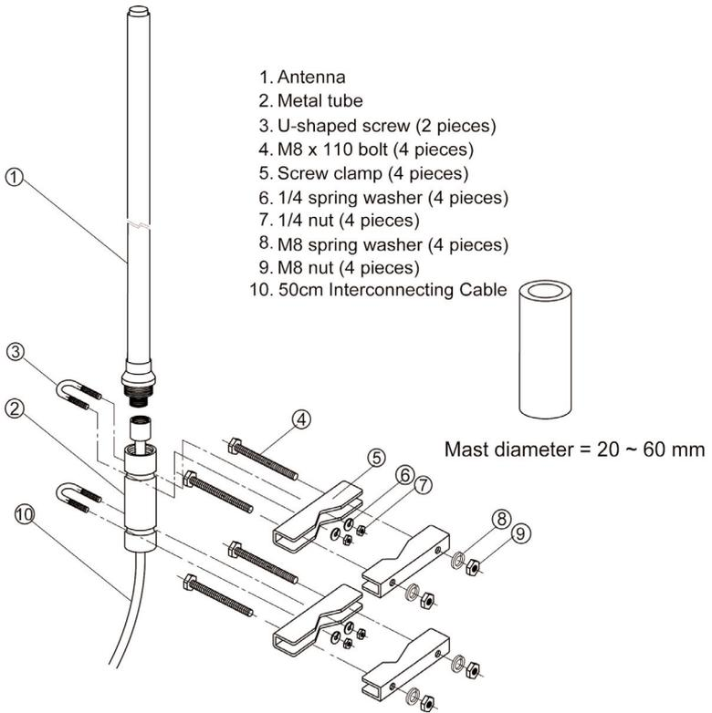
**Figure 3-1. Using the included components to install the LW6200A.**
