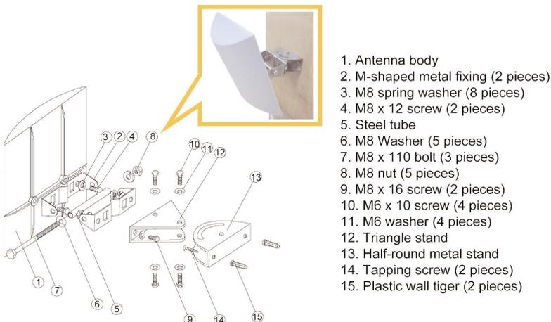
**Figure 3-2. Using the included components to install the LW6201A.**
