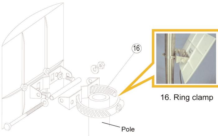
**Figure 3-3. 14-dBi Directional Panel Antenna mounted on a pole, secured with a ring clamp.**
