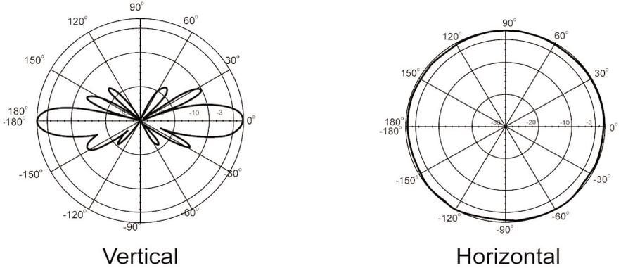
**Figure 1-1. LW6200A's radiation pattern.**
