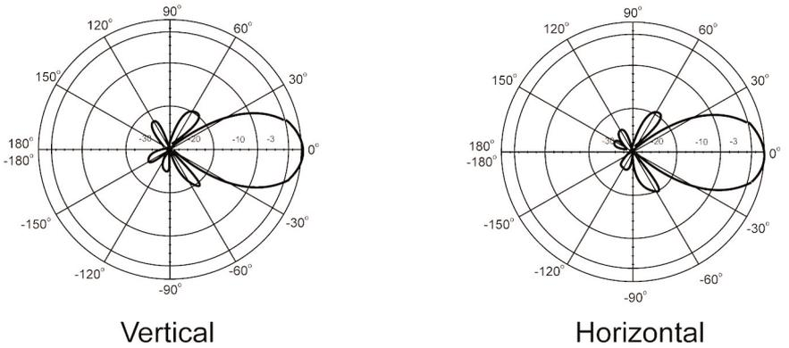
**Figure 1-2. LW6201A's radiation pattern.**
