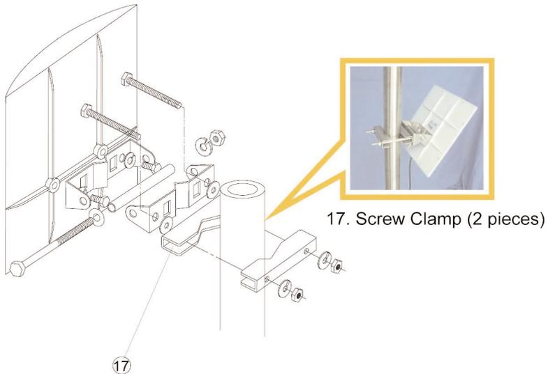
**Figure 3-4. 14-dBi Directional Panel Antenna mounted on a pole, secured with a screw clamp.**
