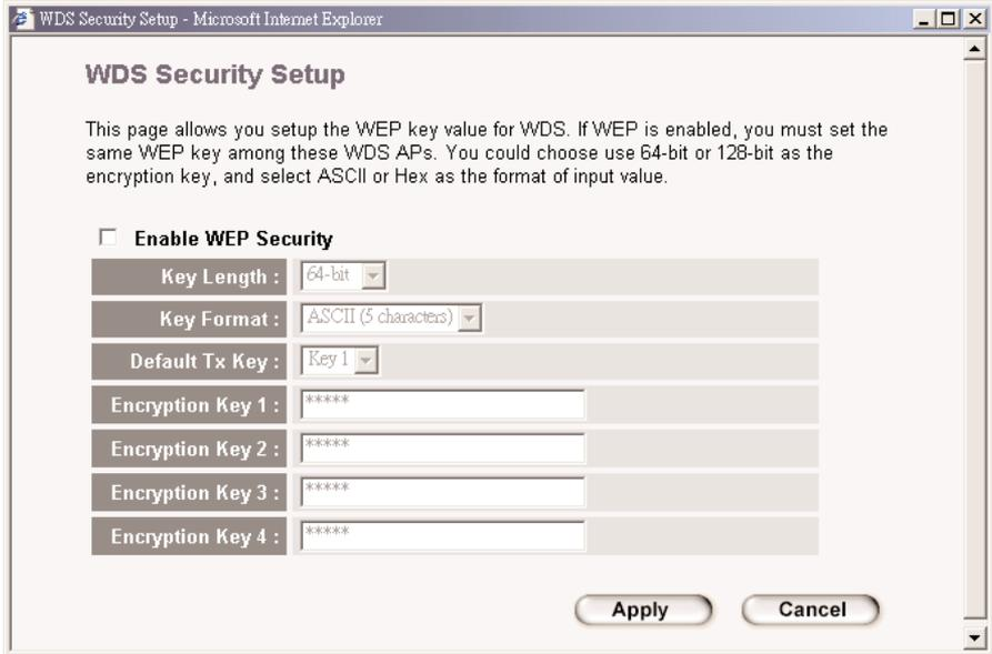
Figure 5-18. WDS security setup screen.
