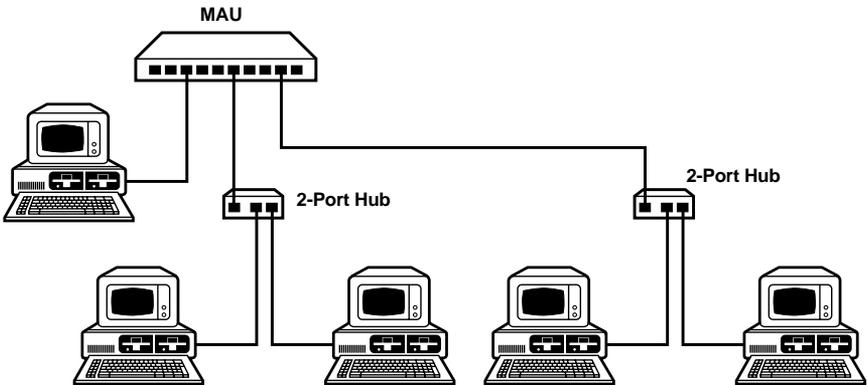
**Figure 2. A Typical 2-Port Hub Application.**
