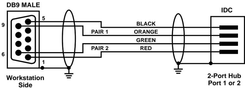
Figure 8. Workstation to 2-Port Hub Connection for STP.
