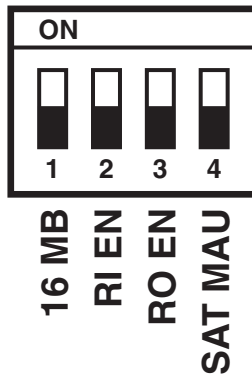
Fig. 3-1. Front-Panel DIP Switch Selections.
